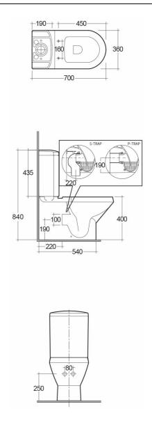
Dimensions: All dimensions in mm tolerance ±5% for below 200mm and ±3% for above 200mm.
