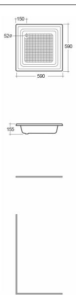
Dimensions: All dimensions in mm tolerance ±5% for below 200mm and ±3% for above 200mm.
