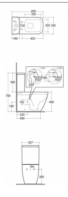
Dimensions: All dimensions in mm tolerance ±5% for below 200mm and ±3% for above 200mm.
