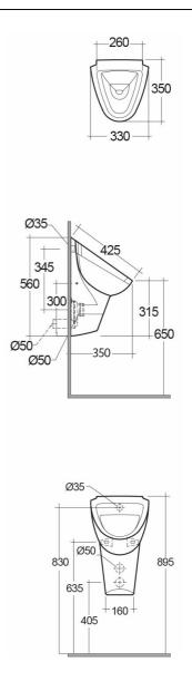
Dimensions: All dimensions in mm tolerance ±5% for below 200mm and ±3% for above 200mm.
